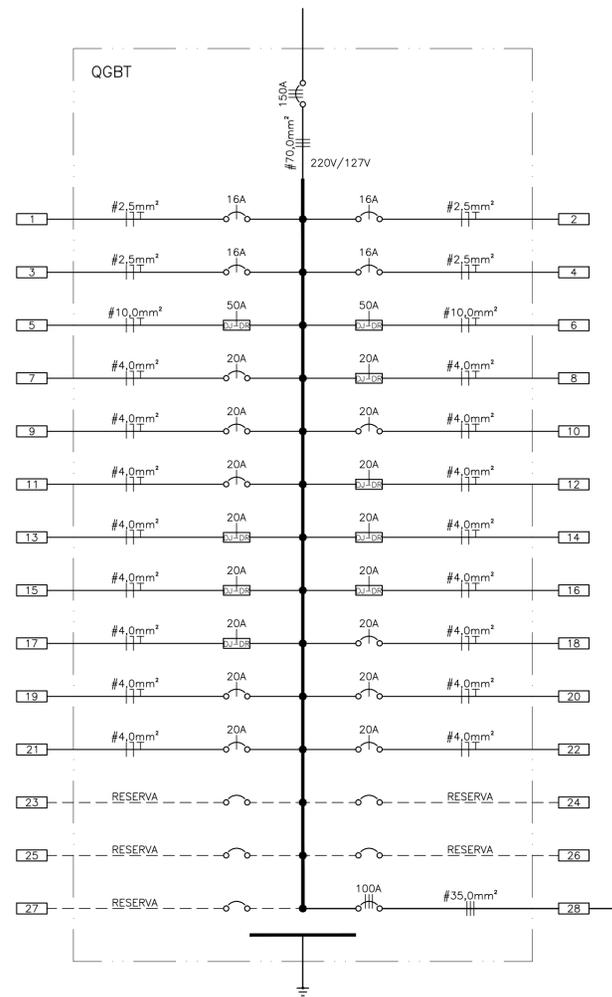
**1** DIAGRAMA UNIFILAR QGBT – PAV. TÉRREO
